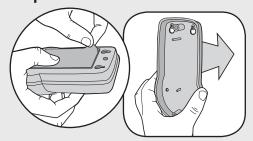
Peel paper from mounting tape. Firmly press Outdoor Intercom onto mounting surface.
